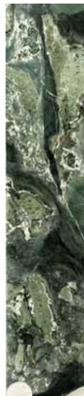
Figure A-1. Drill core sample from the Turner-Albright mine showing siliceous argillite that is interbedded with lavas of the Josephine ophiolite. The black and green laminations are interpreted as terrigenous and tuffaceous in origin, respectively. The alternating black and green colors are also typical of the hemipelagic sequence overlying the Josephine ophiolite. Note coin for scale.
