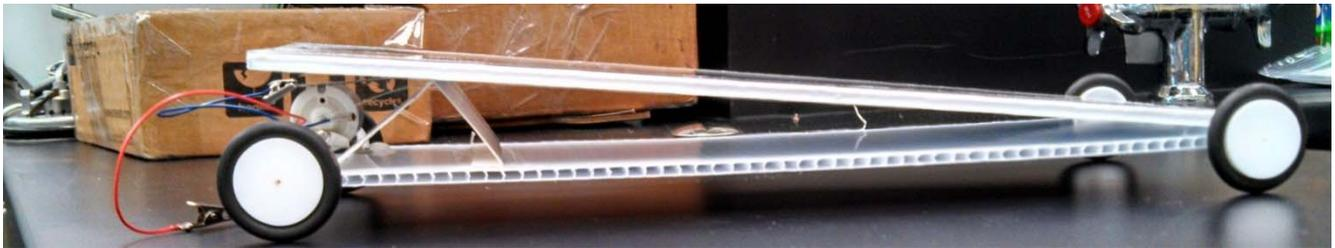
The rubber rings are placed over the wheels to serve as tires, as shown, and the wheels are mounted on the axles.
