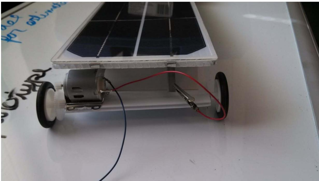
The motor mount can be simply glued to the cardboard base as seen here. Screws can be used if the team prefers a more secure attachment.
