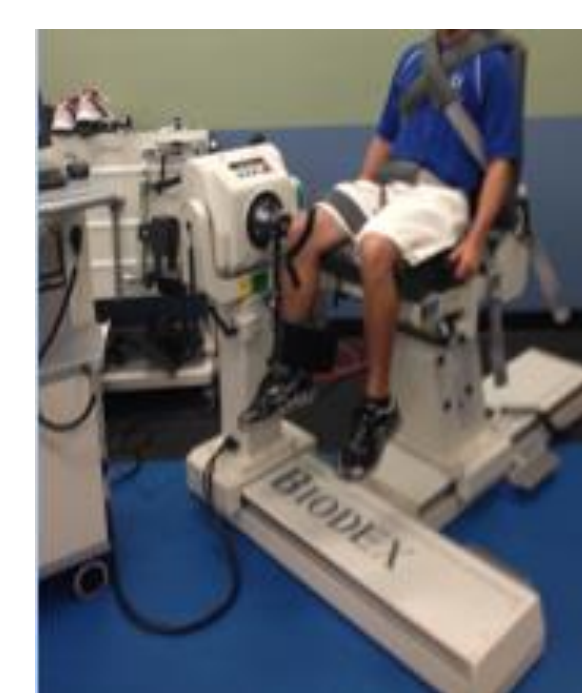
FIGURE 1. Biodex set up for testing of rectus femoris muscle
